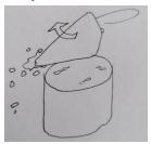
Auger sampling of 0–10 cm layer for chemical analysis 5–20 x cores in one polyethylene bag per permanent plot
